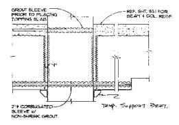
This detail drawing of the Emerson House framing system shows a typical momentframe precast joint.
